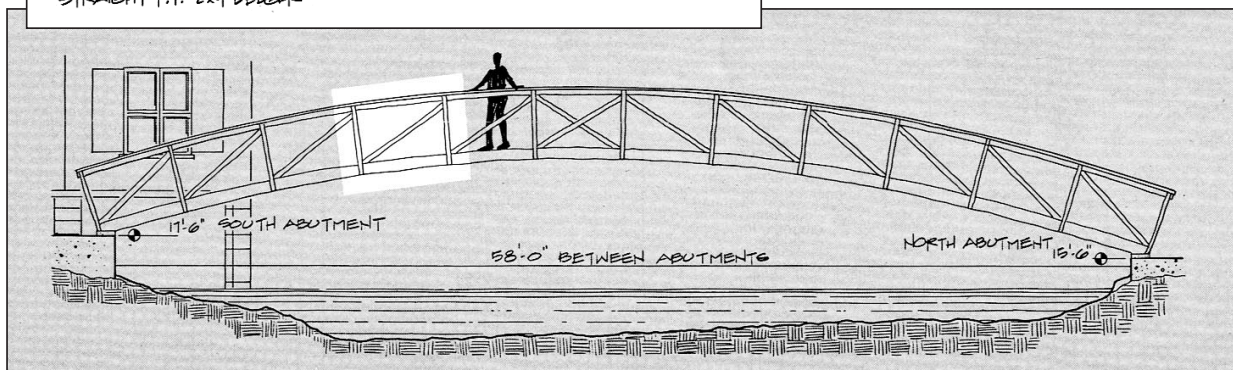
Though the idea of a single 58-foot span initially caused some safety concern, Hyman said the bridge is engineered to support the entire third and fourth grade classes from the local elementary school.
