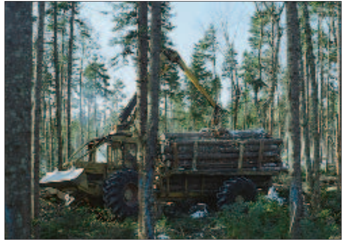
Seven Islands' Scandinavian logging techniques minimize soil damage and allow selective cutting. A processor (left) cuts and trims individual trees. The forwarder (right) carries logs away rather than dragging them.
