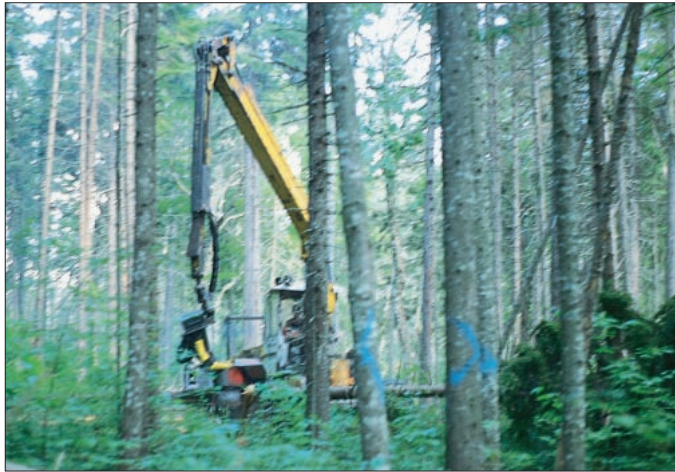
Seven Islands' Scandinavian logging techniques minimize soil damage and allow selective cutting. A processor (left) cuts and trims individual trees. The forwarder (right) carries logs away rather than dragging them.
