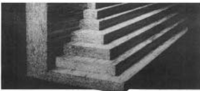
Parallam—soon to be introduced—is made from long, skinny strands of wood glued together. The lumber is strong and stiff, and has a distinctive grain pattern.
