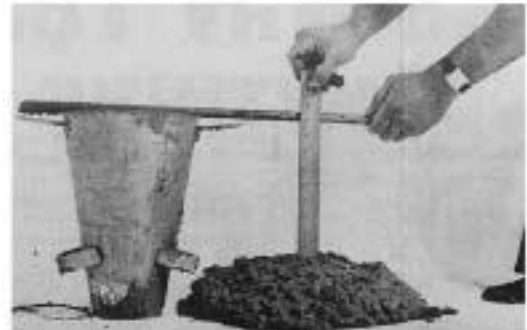
Superplasticizers turn the stiff mix (above) into the easily worked high-slump mix (below) without reducing strength or increasing shrinkage cracking.
