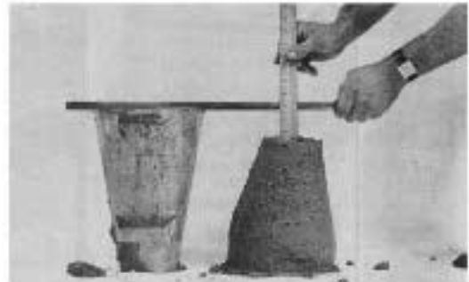
Superplasticizers turn the stiff mix (above) into the easily worked high-slump mix (below) without reducing strength or increasing shrinkage cracking.
