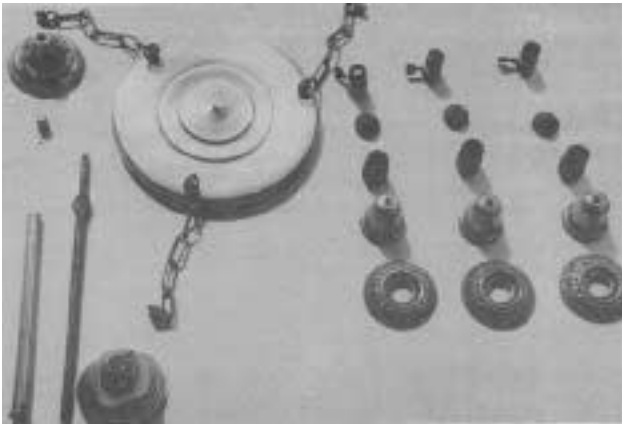
An old three-light chandelier, disassembled and cleaned. At left from top to bottom is the filial, spine with screw-on connectors, and ceiling pan. Toward the center is the main part of the chandelier, with chains and screw-on mounts for the socket assemblies. At right are three socket assemblies. From top to bottom each has socket, metal socket top, paper insulator, metal body for the socket, decorative ring.
