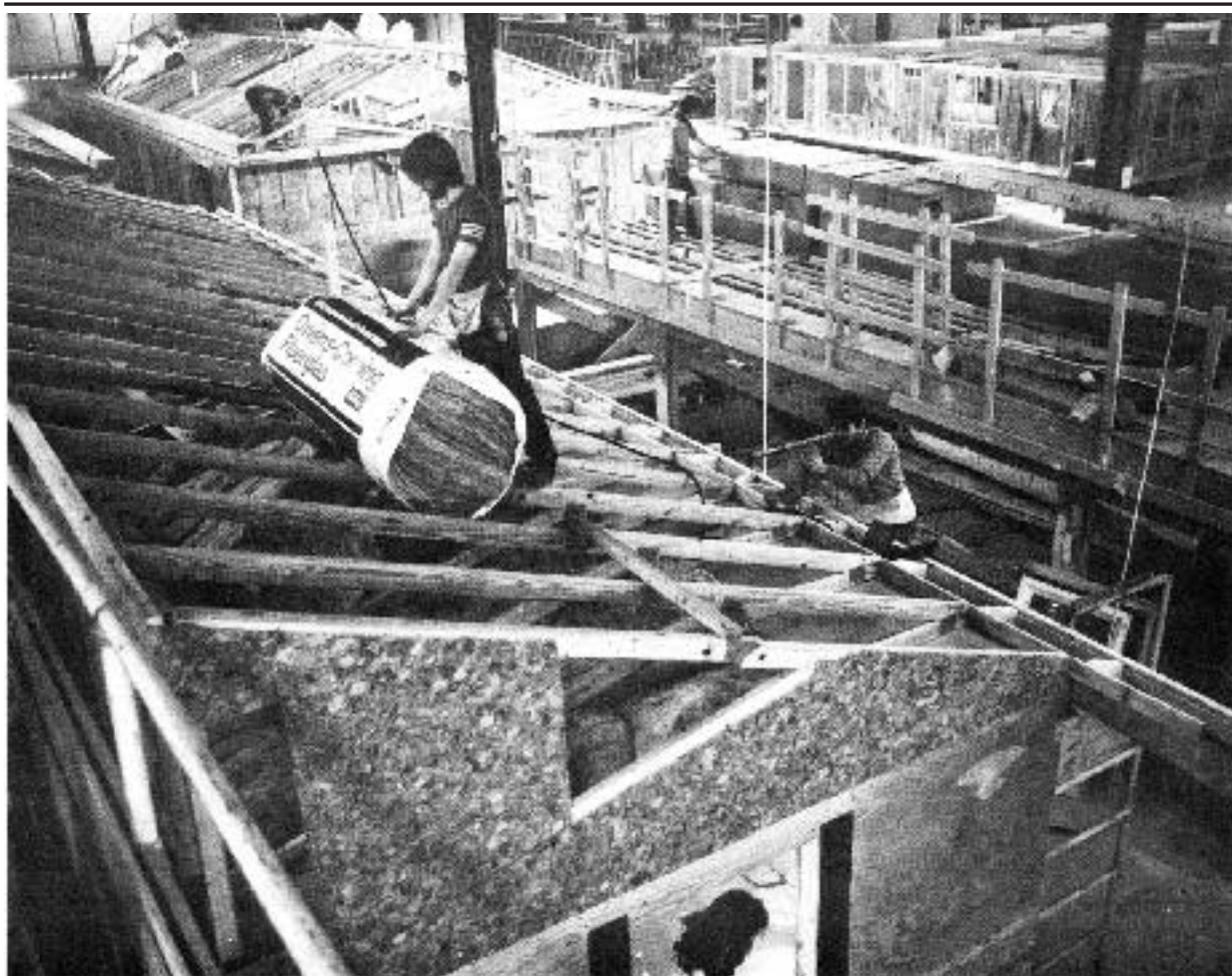
At many home factories, the workers stay in one place and do one job, while the homes move through the factory. Because it's under a roof, work such as insulation can be installed from the exterior.
