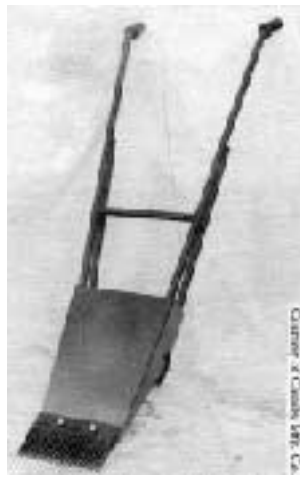
Figure 3. This wheeled tear-off bar can be used to remove shingles or built-up roofing. While it can't compete with the gas and pneumatic machines used to strip big commercial roofs, it has lots of advantages over a hand spud bar and costs less than $200.
