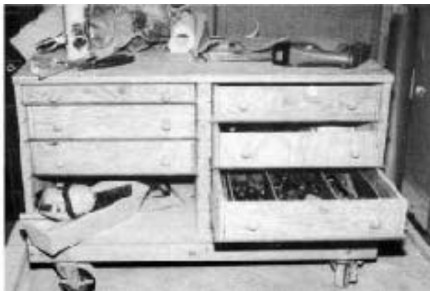
Figure 3. Everything's on wheels. At left, the rolling trolley can carry slat-wall panels and tools. At right, the gang box holds tools and equipment.
