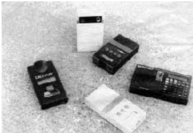
These devices reflect sound waves off surfaces to measure distances. They are not accurate enough for either framing or finish work, but they are useful for estimating. Shown here (clockwise from left), are the Digitape, the Sonin 250 target and transmitter, the Dimension Master Plus, and the Sonin 30.
