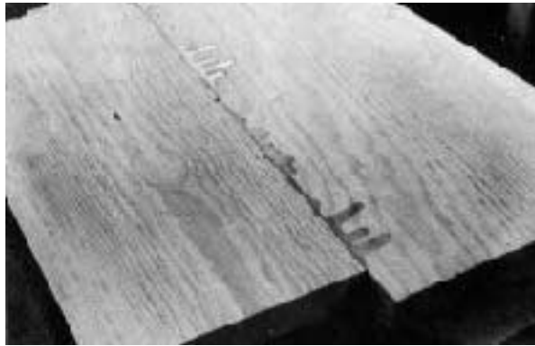
Figure 3. Many glues make finishing difficult if they squeeze out of the glue joint. This is not a problem with liquid hide glue, which washes out of the wood pores, but hide glue dries slowly and requires clamping.
