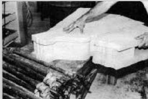
Figure A. Built-up moldings benefit from a waterproof adhesive. This worker is gluing the last piece in place with a waterproof PVA (yellow) glue. The assembly will be clamped until the glue dries.
