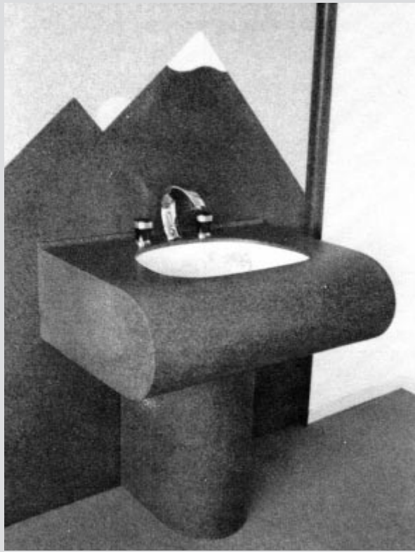
The curved front of this vanity is made of 1/2-inch Corian heated to 325°F and postformed. The sink, also Corian, is seamed from beneath. The mountainscape in the background was created with careful router work and different colors of Corian.
