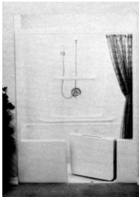
Figure 2. This accessible design from Bathease includes a hinged "door" that relies on the water pressure inside the tub, and an inflatable gasket, to keep water in.
