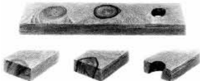
Figure 2. In the grading process, knots are judged either sound or unsound. Sound or "tight" knots, at left, are intergrown and will not fall out. "Encased" knots, center, are allowed in lower grades, but cannot be counted on to stay put, right.
