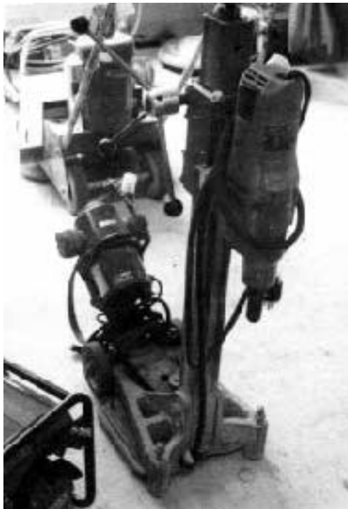
A core drilling rig — a portable drill press that bolts to a slab or wall — can drill holes up to 18 inches in diameter.
