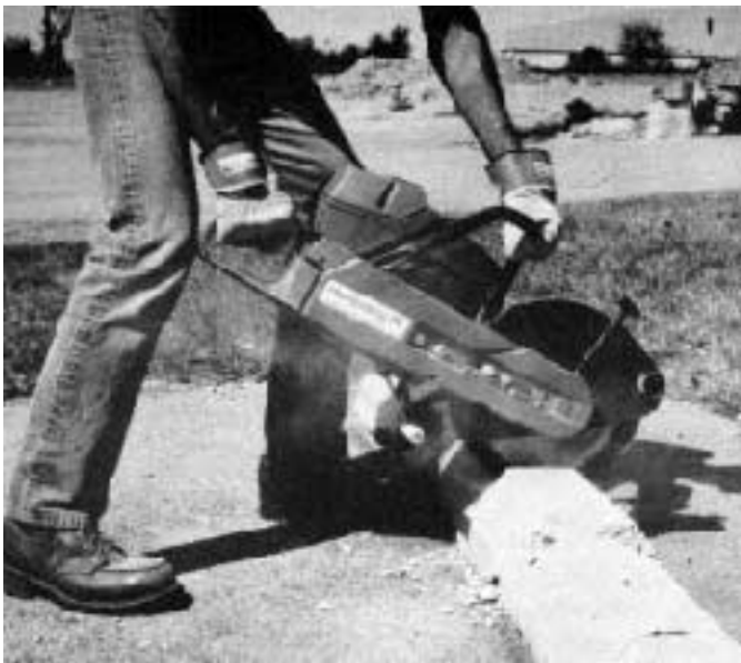
Gas-driven cutoff saws have more power than the electric models, but are noisy, and the dust and exhaust make them unsuitable on many remodel jobs.
