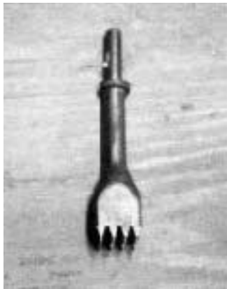
A bushing tool is good for roughing up concrete.
