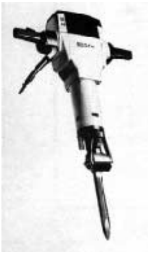
An electric jackhammer has less striking force than a pneumatic or hydraulic hammer, but is easy to rent because it doesn't require a compressor or hoses.
