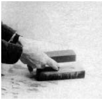
Figure 2. When honing the blade, maintain the angle of the bevel by holding the tool with the forefinger of one hand running down the side of the blade, and the fingers of the other hand gently pressing on the back of the blade. Keep your wrists locked and let your arms do the work.
