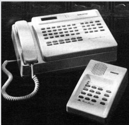
Figure B. The Samantha system combines X-10 control with a touch-tone phone, intercom, and answering machine.
