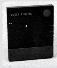
Figure C. With its voice-activated controller, the Butler-in-a-Box is ideal for handicapped persons. It controls lights and appliances through X-10 technology.
