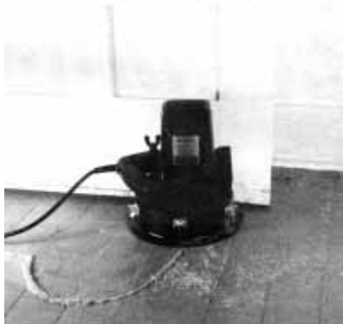
Figure 2. With the Super Saw, doors can be undercut while still hanging in place. The blade housing will adjust up to 1 1/4 inches, which is enough height to undercut a door half an inch before 3/4-inch flooring is installed.
