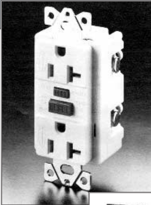
Residential ground-fault circuit interrupters are available in two types. Use receptacle-style GFCIs where possible for convenient resetting at the point of use. GFCI circuit breakers (inset) protect an entire circuit but must be reset at the panel.
