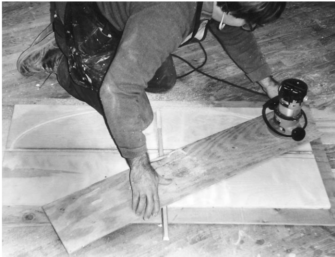
Grant Taylor of South Ackworth, N.H. hogs out a perfect ellipse with his router as he builds an elliptograph — a shop-made jig for cutting an ellipse. When he is finished making the jig, Taylor will use it for making precise cutouts for custom door lights, elliptical arches, and oval sinks.
