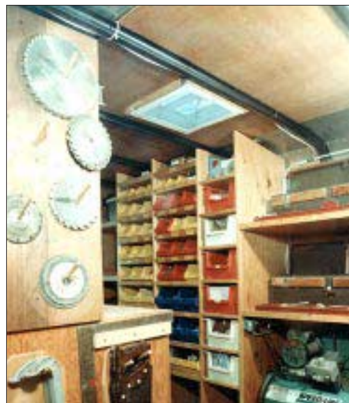
The finish trailer has bins for the many small pieces of hardware needed to finish a house, as well as toolboxes full of hand tools. The air vent in the ceiling provides summertime ventilation and much needed light to the dark interior.
