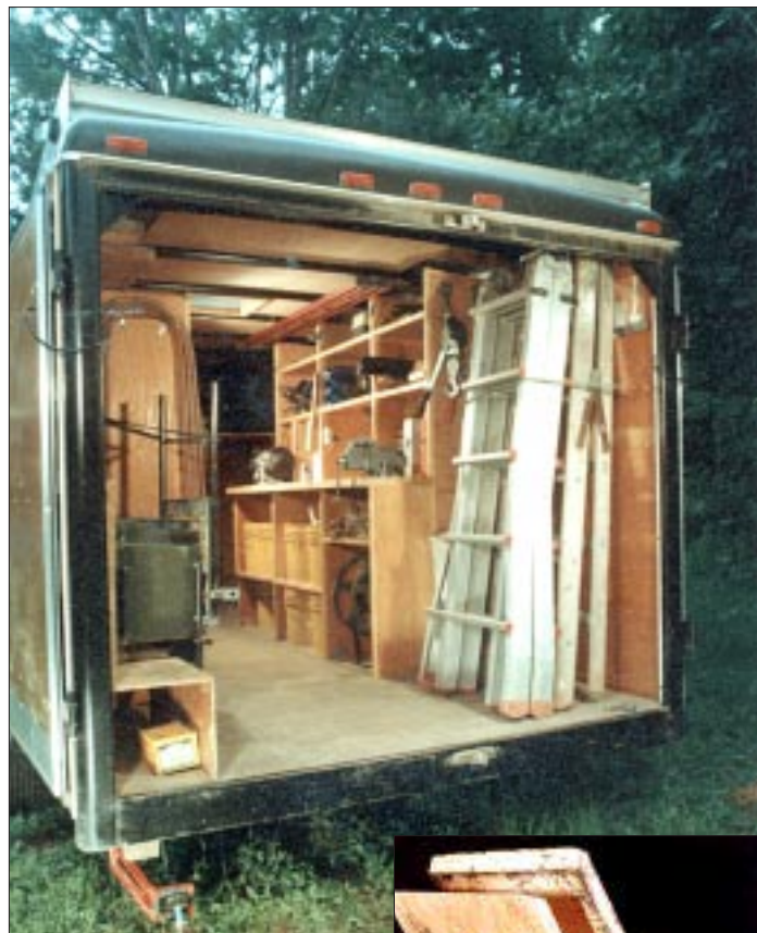
The framing trailer is loaded with standard carpentry tools for a framing crew, including a contractor's table saw (on its side, at left) and a two-horse compressor. The air hose — 300 feet of it — feeds from its reel along the underside of the trailer to a removable guide arm extending from the end (inset).
