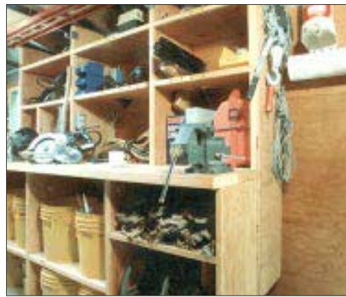
A workbench along one side of the framing trailer holds a heavy-duty vise and a grinder, with bucket storage underneath and tool cubbies above (left). On the other side, bins hold frequently used hardware and a large reel holds the air hose (below, left).
