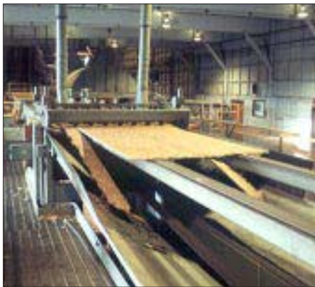
Figure 1. Top: A hopper full of strands that will be pressed into plies. Above: The edges of a completed OSB panel are trimmed as it rolls out of the press.
