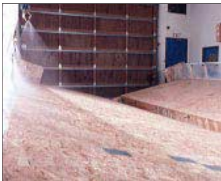
Figure 2. To qualify for the APA stamp, a mill's samples must pass a battery of tests. Top: A wall sheathed with OSB is subjected to increasing racking pressure to measure deflection and ultimate failure. Above: OSB panel undergoes a three-day soak before structural testing.
