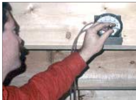
Figure 3. A flow station (left) and magnehelic gauge (center) are used to measure air flow and static pressure in the duct system. To balance the intake and exhaust sides, the installer adjusts in-line dampers (right).
