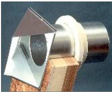
Figure 2. The author uses double-ducted collars (left) to seal the outside vapor barrier of insulated flex duct to the exterior intake and exhaust hoods. He applies a bead of sealant around the collar before attaching it to the band joist (right).
