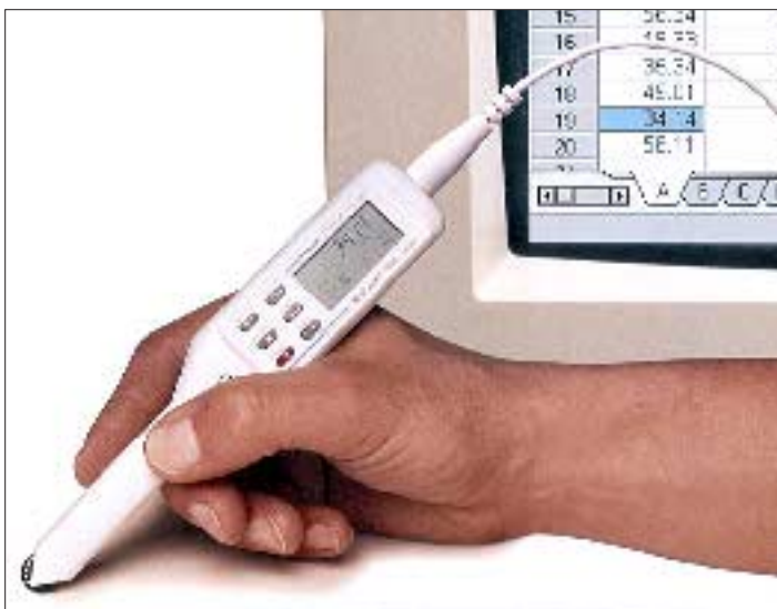
Figure 1. The Scalex works like an electronic planimeter. As you roll the wheel over a set of plans, the stylus electronically translates the travel distance into a dimension, which is displayed on the built-in LED. The Scalex can also be hooked to a computer, and works with several estimating programs and spreadsheets.
