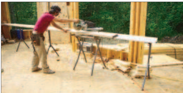
Suitable for framing and finish work, the Saw Helper miter saw stand features rugged aluminum table extensions with adjustable legs and built-in tape measures (left). The whole rig knocks down quickly for easy transport and storage (right).
