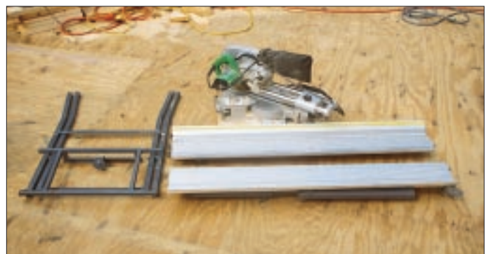
Suitable for framing and finish work, the Saw Helper miter saw stand features rugged aluminum table extensions with adjustable legs and built-in tape measures (left). The whole rig knocks down quickly for easy transport and storage (right).
