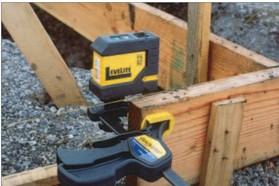
The LeveLite self-leveling laser works more like a plumb bob than a traditional level. A laser diode hangs from a short pendulum inside the case and projects a light beam perpendicular to the pendulum arm to find level.
