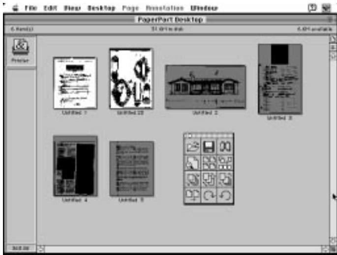
Figure 2. PaperPort displays scanned images as "thumbnail" sketches. In the Macintosh version shown here, images can be grouped and filed in separate folders, and enlarged to full size for viewing.
