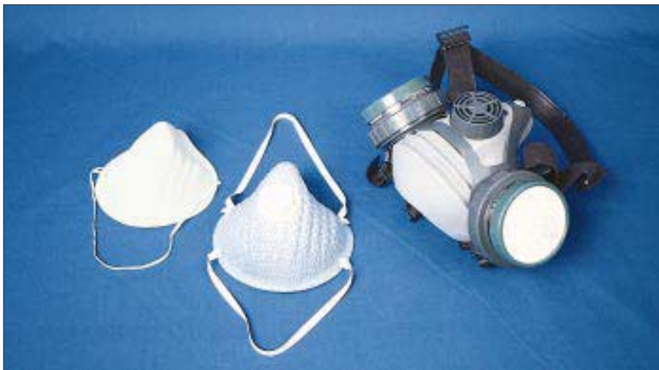
Figure 3. To protect your lungs, assess the hazard carefully. A nuisance dust mask (left) might be fine for a few minutes of demolition, but anyone working in dust all day should have a better fitting dust mask (center) or a respirator with appropriate cartridges (right).
