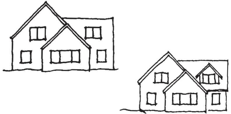
Avoid flat-roofed additions — they conflict visually with existing sloped roofs (left). A sloped-roof solution can usually be found (right).
