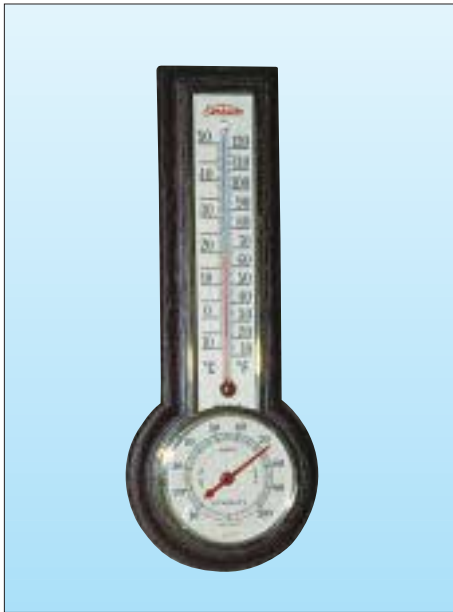
Tools of the finisher's trade. The author uses two diagnostic tools on every job: a combination thermometer/hygrometer (left) and a moisture meter (right) to measure the wood flooring's moisture content. If conditions are not within the proper range, the finish may fail.
