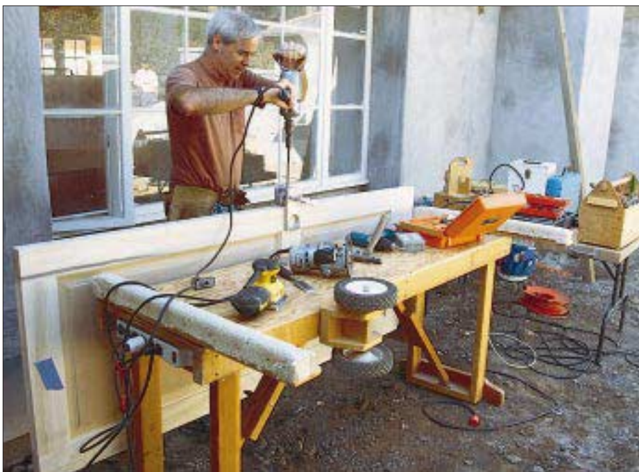
Door hanger's bench. Robert Brown wastes little time mortising for hinges and boring for locksets with this simple, elegantly designed workbench. His rig also serves as an easy-to-transport saw stand and work table.
