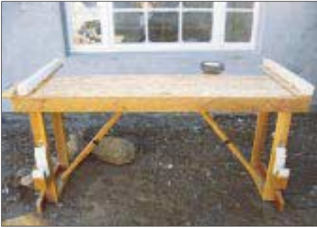
Figure 1. The crossarms on top of the bench are designed to support a door lying flat. When used as a miter saw stand, the crossarms serve as stock supports.
