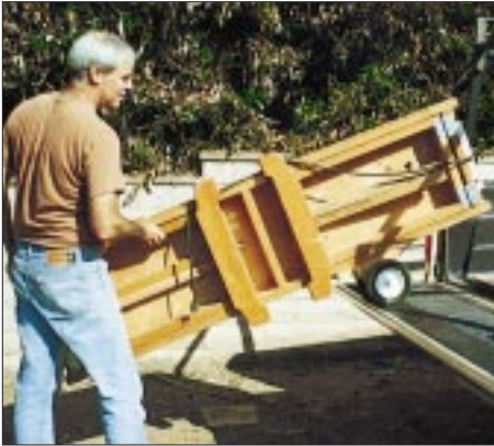
Figure 2. Wheels make it easy for Brown to move the bench in and out of the truck.
