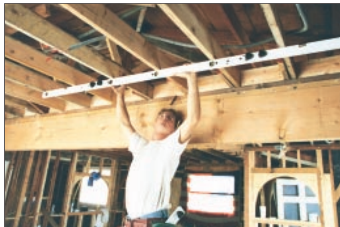
Figure 2. A carpenter uses the Levelution in 8-foot mode. The triangular knobs mark the joints in this expandable rail. A 1-foot accessory (visible in the carpenter's pocket) can be swapped in at any joint to make levels of other lengths.
