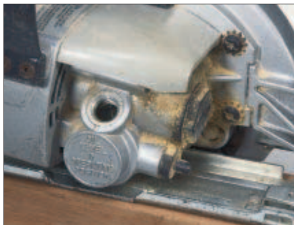
Figure 4. Wormdrive oil check. Wormdrive circular saws have an oil bath that lubricates the gears. To check the oil level, set the saw at maximum cutting depth and put the shoe flat on a benchtop. Remove the oil filler cap. The oil should be right up to the edge of the opening.
