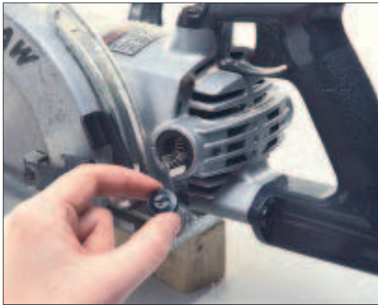
Figure 2. Wormdrive brush replacement. Remove the brush holder covers to access the spring-loaded brushes (left). Check both brushes during maintenance, because they may wear at uneven rates. Always replace both at the same time. When inserting the new brushes (below), be careful not to get any oil or dirt on the brush, spring, or housing.
