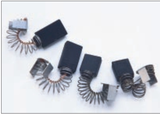
Figure 1. Brush inspection. The used brushes, at right, are clearly shorter than the new ones. A general rule is to replace brushes when they wear down to 1/4 inch. However, the ones shown here should be replaced because of the damaged spring on the brush on the far right.
