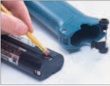
Figure 5. Battery cleaning. The metal contacts on the batteries of cordless tool systems need to be clean to transfer electricity efficiently. A pencil eraser works well to rub off any gunk that has built up. If they are accessible, clean the contacts inside the drill handle and the charger as well.
