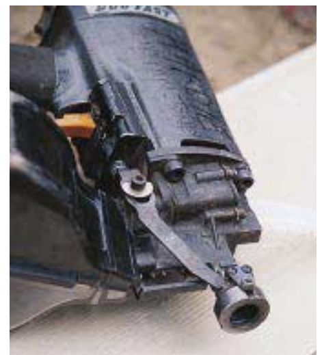
Figure 3. It's important not to overdrive fasteners in fiber-cement, which is why it's a poor idea to apply it with framing guns. Coil nailers do the job more accurately, especially if they have a mechanism for adjusting depth-of-drive, like this after-market retrofit tip from Duo-Fast.
