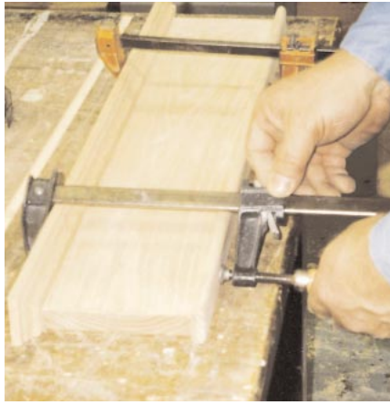
Figure 3. Ulmia spring clamps help in gluing up return miters on the cap moldings (left). The three pieces of the head trim are glued together to form a single piece (right).
