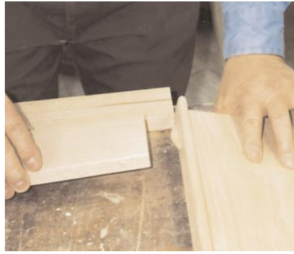
Figure 5. Once the head trim is assembled, the author biscuit-joins the side casings to the head piece. He clamps the pieces to a backer piece to make sure the back is perfectly flat.
