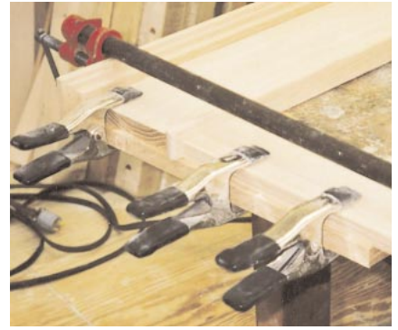
Figure 5. Once the head trim is assembled, the author biscuit-joins the side casings to the head piece. He clamps the pieces to a backer piece to make sure the back is perfectly flat.
