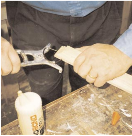
Figure 3. Ulmia spring clamps help in gluing up return miters on the cap moldings (left). The three pieces of the head trim are glued together to form a single piece (right).
