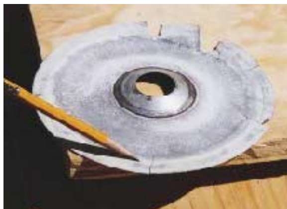
Figure 4. Shown in the top photo are a worn backing pad, flanked by a new pad, top, and a new carbide stripping disc. As soon as discs begin to gum up (middle photo), the author soaks them in stripper. Discs must be regularly inspected for damage. Those with stress cracks (indicated by pencil in bottom photo) are discarded.
