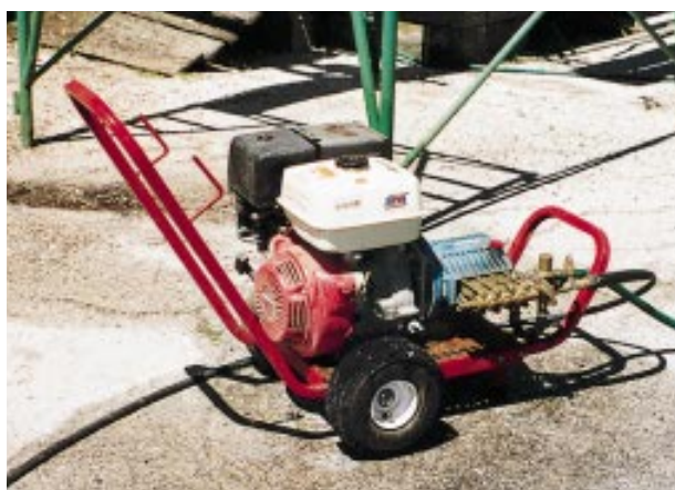
Figure 8. The author uses a 13-horse 3,500-psi Northstar pressure-washer.
