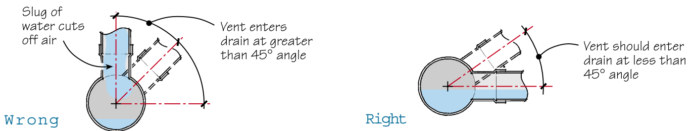
Figure C. Dry vent and wet vent connections to main drain lines are made differently. A dry vent must connect at an angle of 45 degrees or above, measured from a line cut horizontally midway through the pipe. A wet vent, because it carries water and air, must connect at an angle less than 45 degrees to this line.
