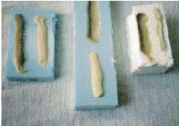
Figure 5. An incompatible construction adhesive (darker bead in photo) will dissolve rigid foam — including poly-faced XPS (on left in photo).
