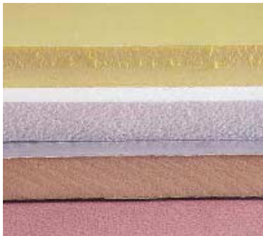
Figure 1. The individual “beads” of foam in expanded polystyrene (EPS) are visible in the rigid blocks or sheets, commonly called “bead-board” (top). Extruded polystyrene (XPS) is uniform throughout its thickness and forms a “skin” while curing, making it impervious to moisture penetration (middle). Polyisocyanurate (bottom) is most susceptible to moisture damage, but has the highest R-value of the three types of foam.
