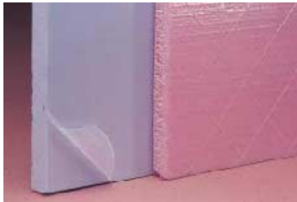
Figure 4. A polyethylene skin, whether plain or reinforced, protects XPS foam from damage during installation and provides a better bonding surface for adhesives. Other facings, such as foil or kraft paper, also serve as radiant barriers, protect against UV degradation, and reduce permeability.
