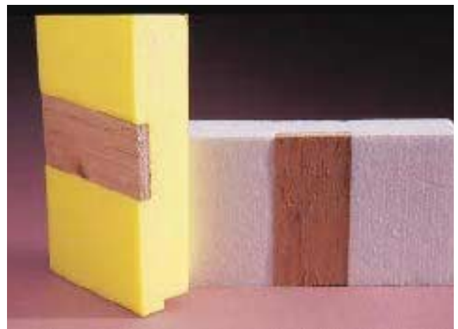
Figure 6. For interior basement insulation, wide shiplaps on some XPS boards accept furring strips, which can be fastened through the foam to poured concrete or masonry (left). Diversifoam's "CertiStud" EPS board has plywood furring strips bonded to the foam (above).
