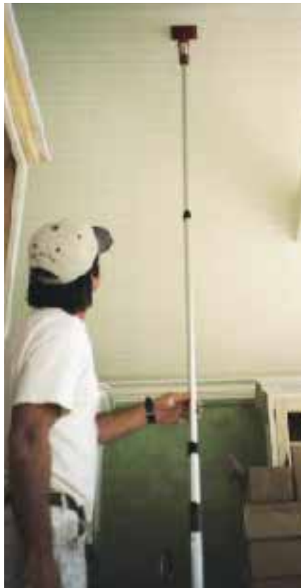
Figure 3. The standard telescoping pole from ZipWall has a 12-foot reach, adjusts easily, and compresses in place to allow the user to trap the bottom edge of the curtain.
