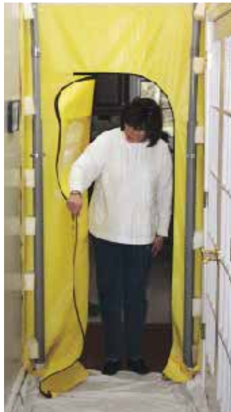
Figure 2. High-quality airtight components and exclusive features like the 4-inch exhaust-duct sleeve make it possible to create a negative-pressure work zone behind the Dust Door.
