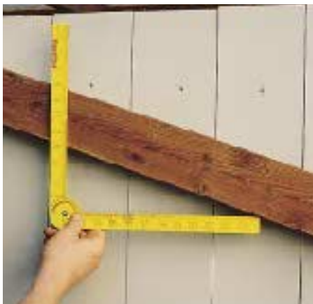
A built-in vial in the RascalRule makes it easy to measure slope in rise/run, percent, or degrees (left). The 2-foot-long folding rule also serves as a bevel gauge and protractor (right).
