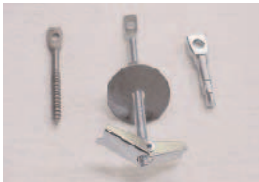
Figure 5. Hanger wires are usually attached to lag eyes driven into ceiling joists. In a concrete deck, "wedgie" anchors are driven into predrilled 1/4" holes. Toggle bolts are the usual choice where it's necessary to place anchors between joists.
