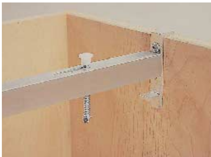
Figure 6. Many undermount sinks, especially large sinks and cast-iron sinks, need to be supported on rails. Vance sells the Sink Undermounter kit, which includes two aluminum rails. The rails have bolts that hold the sink flange against the countertop.
