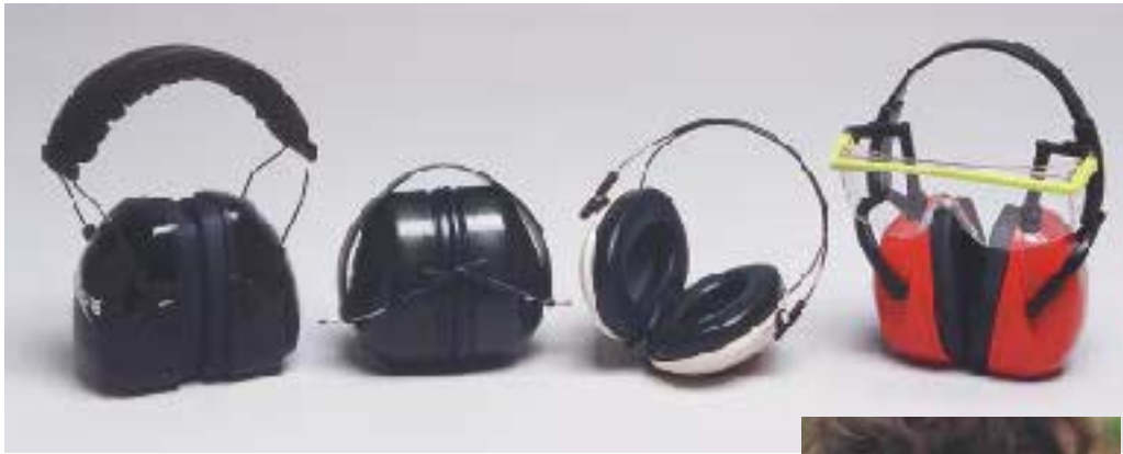
Figure 4. Conventional earmuffs (at left) are comfortable, but bulky. Folding muffs (second from left) fit neatly in a toolbox or the glove compartment of your truck. Behind-the-head style muffs (third from left and inset) can be worn with a hard hat or other headgear, while the OptiMuff (at near right) combines eye and hearing protection in one efficient (if slightly goofy-looking) package.
