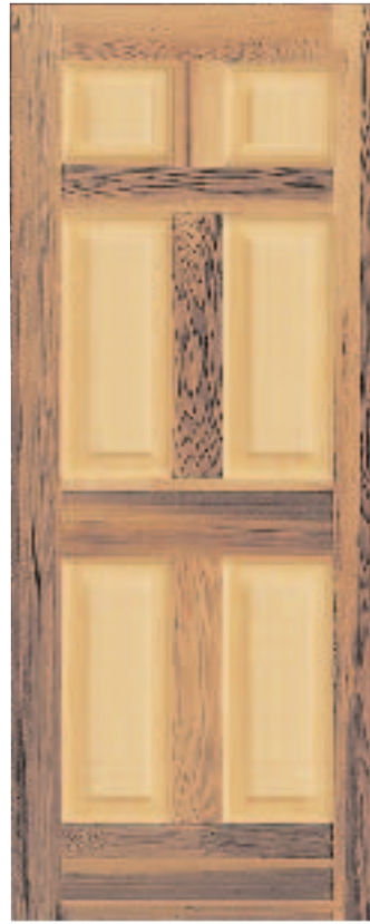
Solid pine panels and a solid cedar frame highlight the classic construction of a frame-and-panel door (left). Select-grade veneer over a core of lower-grade glulam lumber uses lumber economically while producing a more dimensionally stable door (right).
