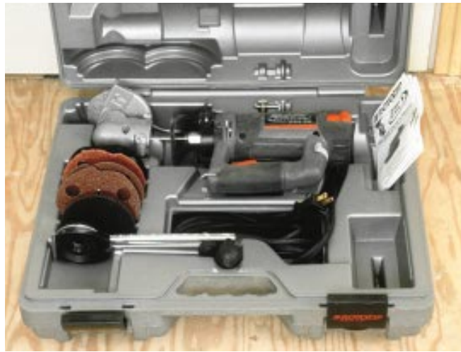
Figure 4. The Revolution Combo Kit includes a circle cutter, a Zip Mate, extra bits, and a plastic case.
