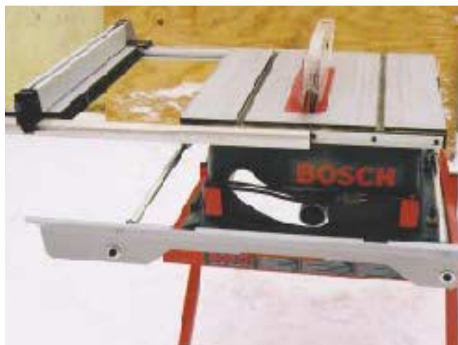
Figure 1. The table extends to provide 25 inches from fence to blade, and an accessory outfeed support adds 18 inches of depth. Note the cord storage lugs on the back of the saw and the molded handgrip on the right side of the tabletop.
