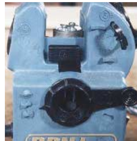
Figure 3. Templates and icons identify point angles (left) and correct settings (right).
