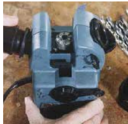
Figure 5. The diamond-coated abrasive cylinder will sharpen carbide bits and is reversible for longer life.
