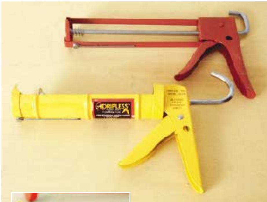
Figure 1. The secret of dripless caulking guns is in the plunger-rod mechanism (inset). Every time you release the trigger, pressure is fully released from the contents of the tube, so the flow stops.
