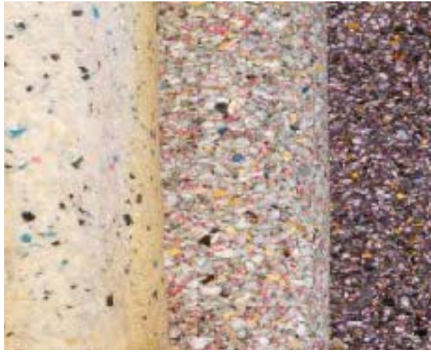
Figure 3. Rebonded urethane foam cushion, made from recycled foam sections, is rated in pounds per cubic foot of density. The denser the foam, the better the “feel” and durability underfoot.
