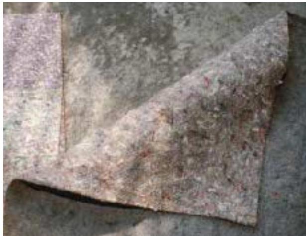
Figure 4. Synthetic felt cushion, made from recycled carpet textile fibers, gives a firm feel underfoot and is typically applied under berber and dense, low-nap, or commercial-style carpeting. Because of its better “breathability,” it’s a good choice for potentially damp concrete basement floors.
