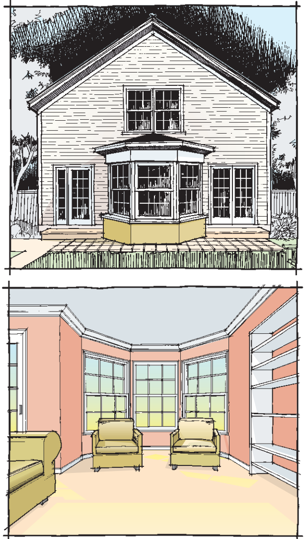
Figure 1. This traditional bay window — part of a proposed addition to the back of a 1948 two-story Colonial revival — is attractive but lacks the visual heft to anchor the new backyard (exterior view). Extending the family room ceiling into the space makes it feel larger, but the angled walls are confining and limit furniture placement (interior view).
