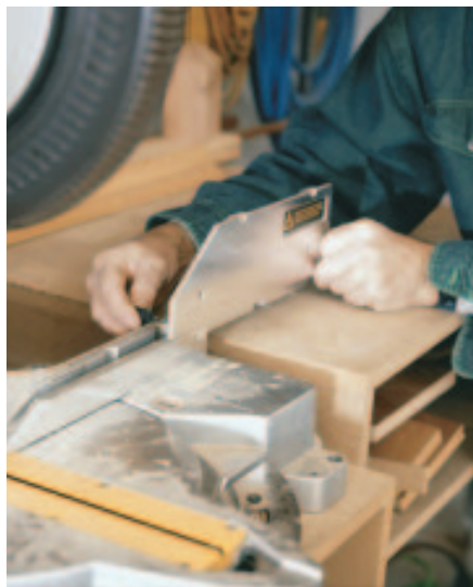
Figure 1. The well-engineered fence allows fast and easy changes from bevel to straight miters.
