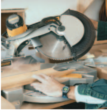
Figure 3. The DW 706 will bevel left and right but still has greater capacity against the fence.
